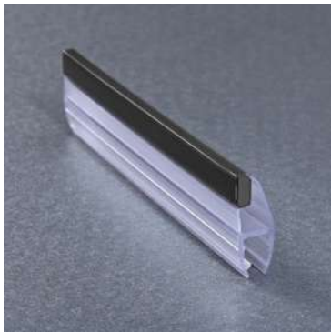
Item No: PS28 Magnetic PVC Seal ▪ Material: PVC ▪ Glass Thickness: 6/8/10mm ▪ Finish:Clear/white/Matte Black
