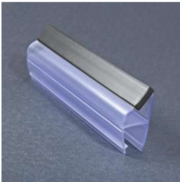
Item No: PS18 Magnetic PVC Seal ▪ Material: PVC ▪ Glass Thickness: 6/8/10mm ▪ Finish:Clear/white/Matte Black
