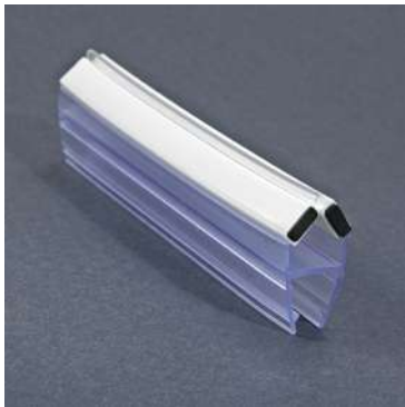
Item No: PS24A Magnetic PVC Seal ▪ Material: PVC ▪ Glass Thickness:10/12mm ▪ Finish:Clear/white/Matte Black
